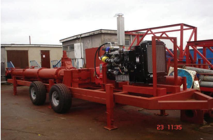
Robust, practical and effective system for crude oil tank sludge recovery through bottom manway access, using Transmas Units and Mastir Cannons. Work using this system has received awards in UK.
